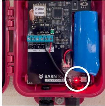
After tapping the pairing button, **if the L2 light flashes Red, then your sensor is NOT Communicating.**
