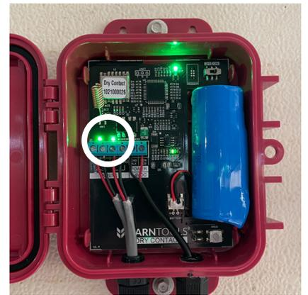
Each input (DIN1 & DIN2) will show you if the WDC sensor is reading an 'Open' or 'Closed' circuit right at the sensor! No need to check the app anymore during this step.
