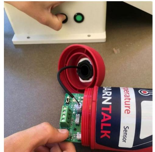
4. Reinstall the sensor cap, tighten until the notches align.
