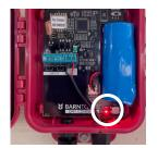
After tapping the pairing button, if the L2 light flashes Red, then your sensor is NOT Communicating.
