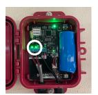
Each input (DIN1 & DIN2) will show you if the WDC sensor is reading an "Open" or "Closed" circuit. No need to check the app anymore during this step.
